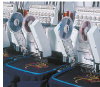
■ Double Sequin Device ● 双侧单珠片装置
