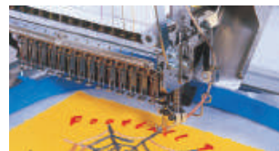
Loop & Cord Device as Cording 当盘带绣装置时，可转为盘带绣
