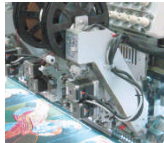
■ Double Twin Sequin Device ● 双侧双珠片装置
